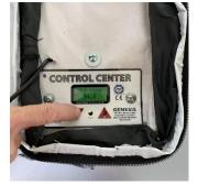
When the heating element is on, the small amber LED underneath the screen will glow.
