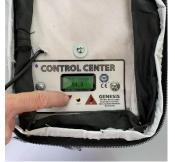
When the heating element is on, the small amber LED underneath the screen will glow.
