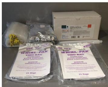
The Aquagenx CBT Kit is the ideal *E. coli* water quality test for on-site testing in-the-field. It is optimized for rural and low resource areas and does not require electricity, labs or expensive equipment. The CBT generates quantified (MPN), color-coded, easy-to-score test results.
