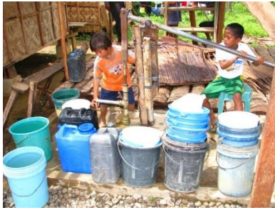
Water collection from a shallow well with hand pump
