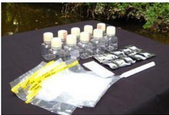
The Aquagenx Compartment Bag Test (CBT) is a portable, simple, self-contained water quality test kit that lets anyone, anywhere determine if drinking water contains *E. coli* bacteria and poses a health risk. No electricity or laboratories are needed. The CBT is ideal for on-site testing in low resource and disaster settings.
