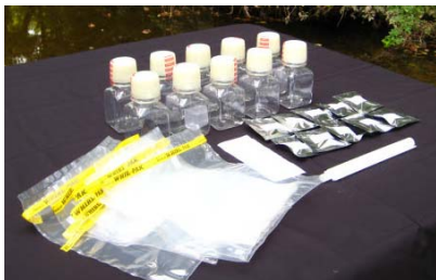
The Aquagenx CBT Kit includes all supplies for field sampling: test bags, sample bottles, growth medium, sealing clip, chlorine tablets for disinfection and instructions.
