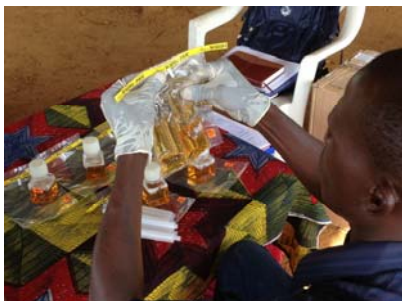
The Aquagenx Compartment Bag Test (CBT) is a simple way to test drinking water for E. coli without the need of a laboratory, electricity or expensive equipment.
