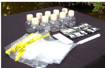
Contract laboratories will typically provide the bottles, coolers and forms needed for compliance monitoring. Or consider using one of the E. coli field tests available for low resource settings.
