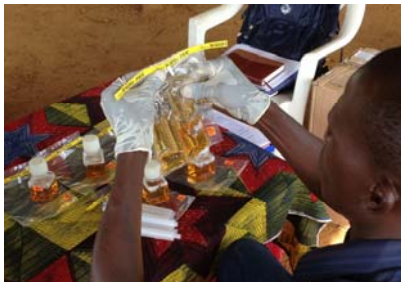
Shown here is the Compartment Bag Test (CBT) by Aquagenx. It is one of the E. coli field tests available on the market. This one requires no electricity or expensive equipment.
